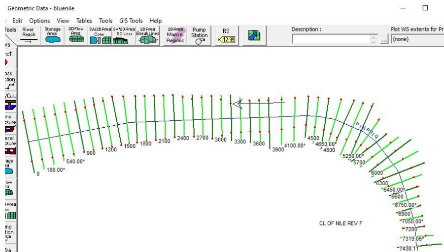
Figure 2: The cross-sections into hec-ras app.
