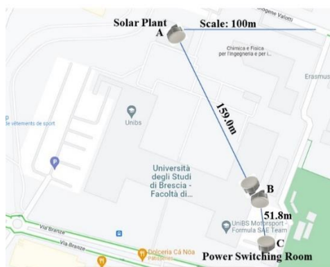
Figure 3: Smart Grid testbed wireless topology.
