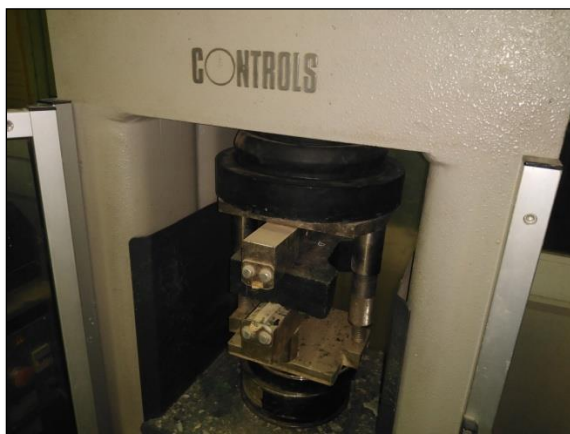
(a) Tested sample on Compressive machine.
