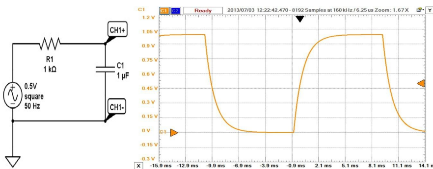
Figure 6 Capacitor Circuit- charge discharge with square wave input
