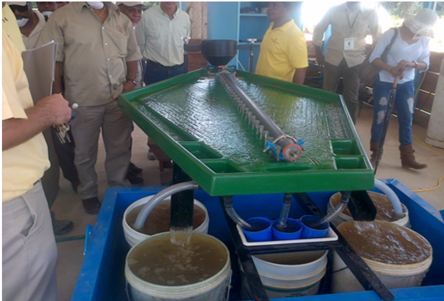
Fig 3; Shaking Table with #1, #2 cups and waste buckets at CMC
