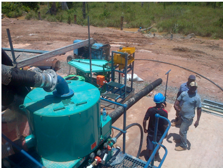
Fig 2: Centrifugal Concentrator and Shaking Table at MCC
