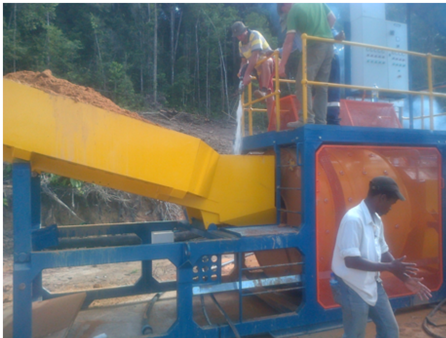
Fig 1: Washing of ore into the Scrubber at MCC
