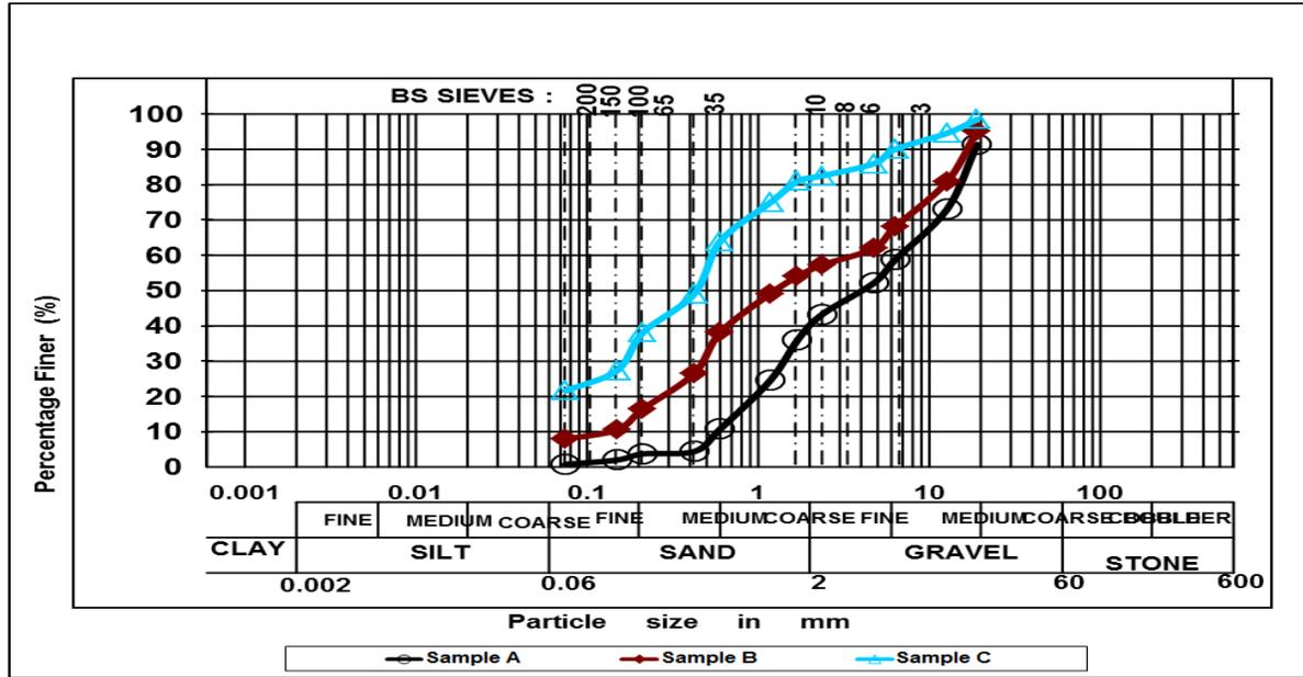
Figure 3: Particle size distribution curves for the MSW samples
