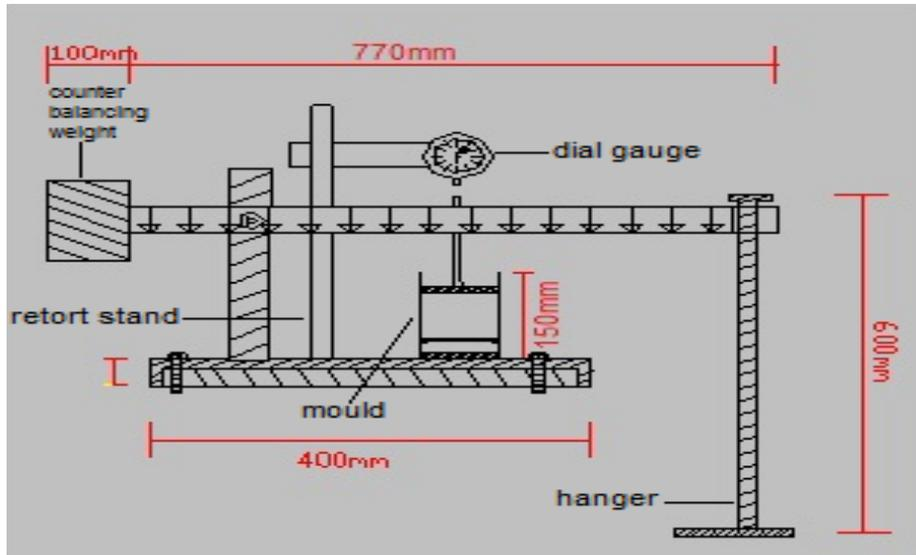
Figure 1: Schematic diagram of the fabricated intermediate scale oedometer experiment set up
