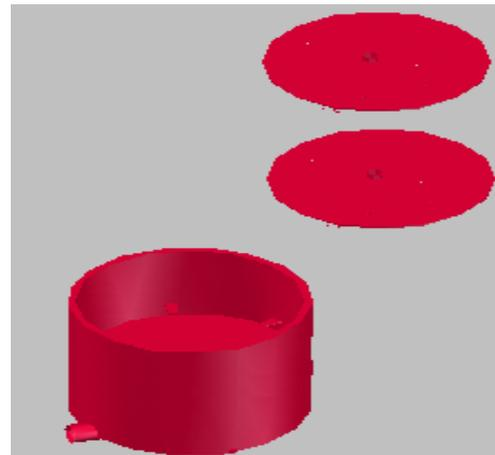
(b) cylindrical mould and porous plates.
