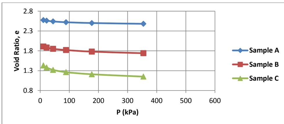
Figure 5: Plot of void ratio vs. pressure for the MSW
