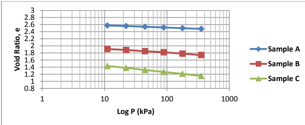
Figure 4: Plot of void ratio vs. log of pressure for the MSW
