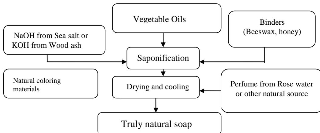
**Figure 2.** Flow process for natural soap making
